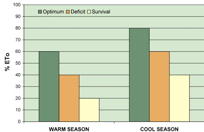
Figure 1. Turfgrass water requirements (as % of ET<sub>o</sub>) at optimum, deficit, and survival levels of irrigation.
