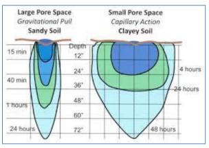
Figure 4 - Comparative movement of water downward and outward in sandy and clay soils Credit: www.ext.colostate.edu/mg/gardennotes/213.html
