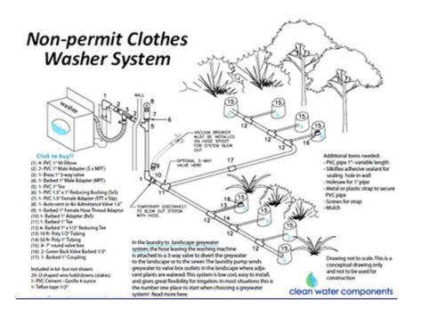
Figure 1 - Diagram of a 'laundry to landscape' graywater system (source: Clean Water Components).
